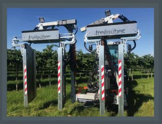
One side in front of the tractor **for pointed lines** to move out of the row.
